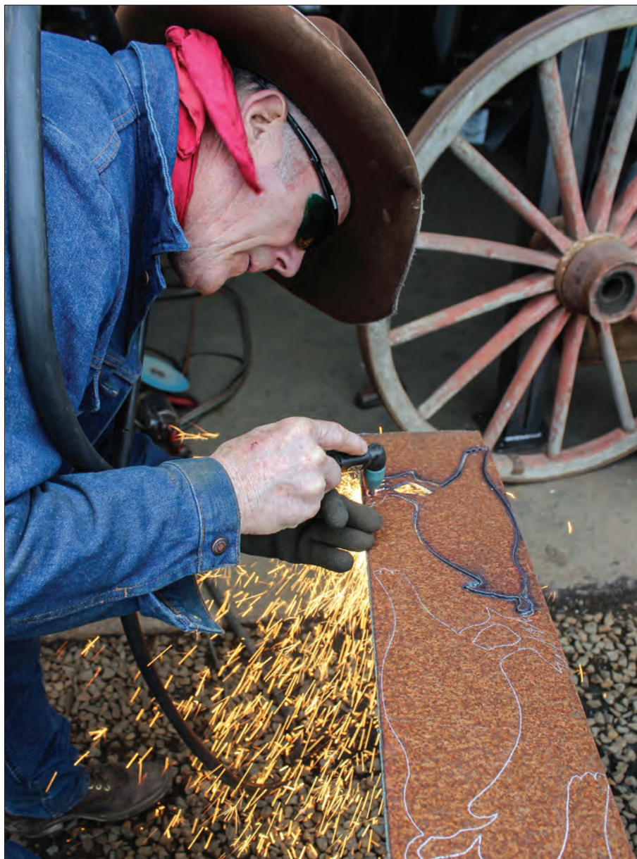
After transferring a design to metal, Wade Skinner cuts the shapes out by hand with a cutting torch.
