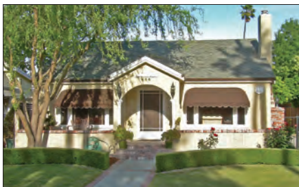
Since most solar gain enters through your home's windows, awnings and shade trees are effective ways to cool your home during summer months.
