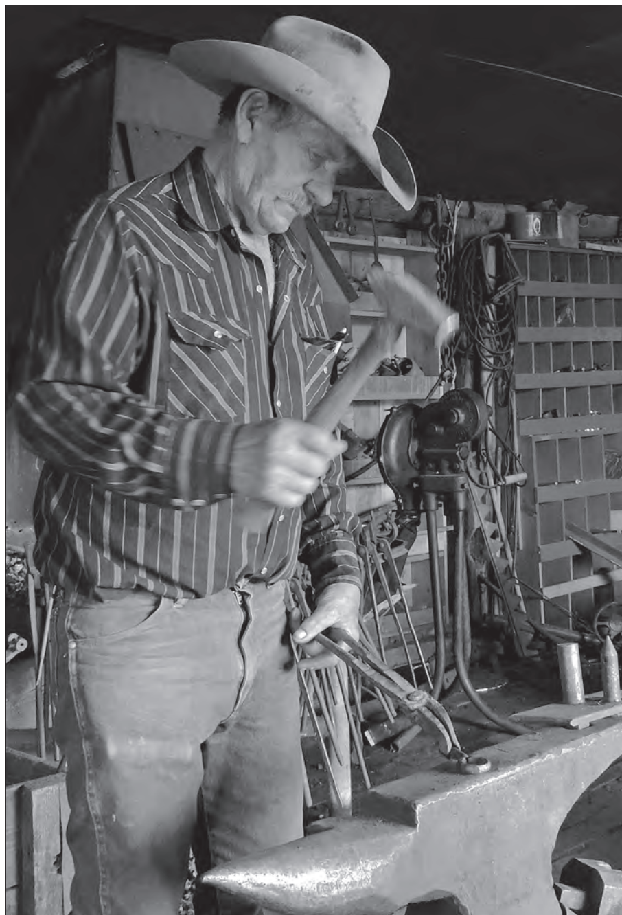
Ray Bagby makes an eye bolt in his blacksmith shop using vintage tools. He has been building vintage horse-drawn vehicles since 1981.
