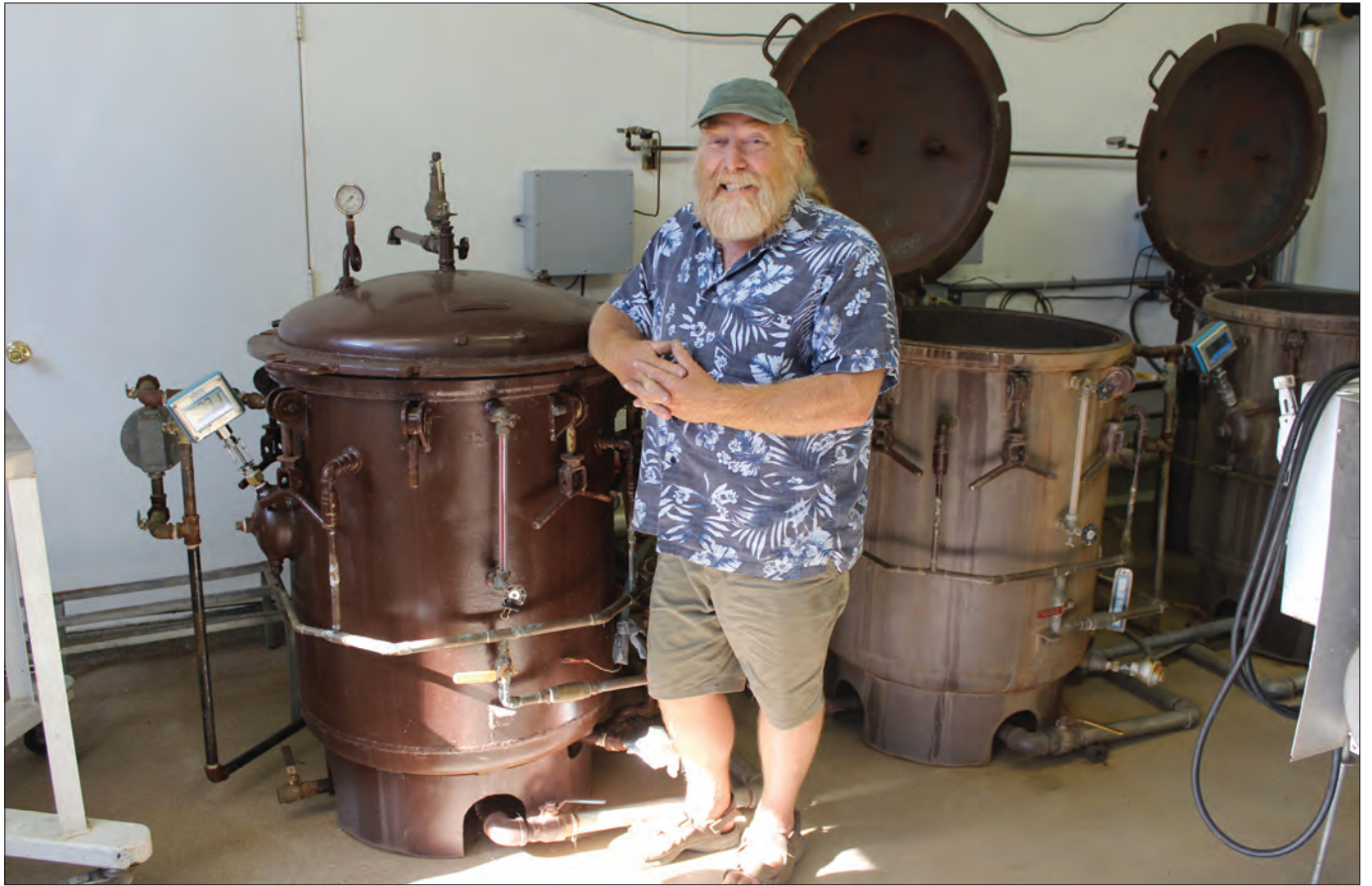
Paul Fuller with his three retorts, which are basically giant pressure cookers. Photo by Craig Reed
