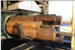
Above, McFarland Cascade Plant Manager Robert Campbell. Left, power poles are fed into a sealed retort, where they are treated under pressure with oil to increase longevity.
