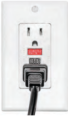
Ground-fault circuit interrupters instantly break an electric circuit when a short develops.
