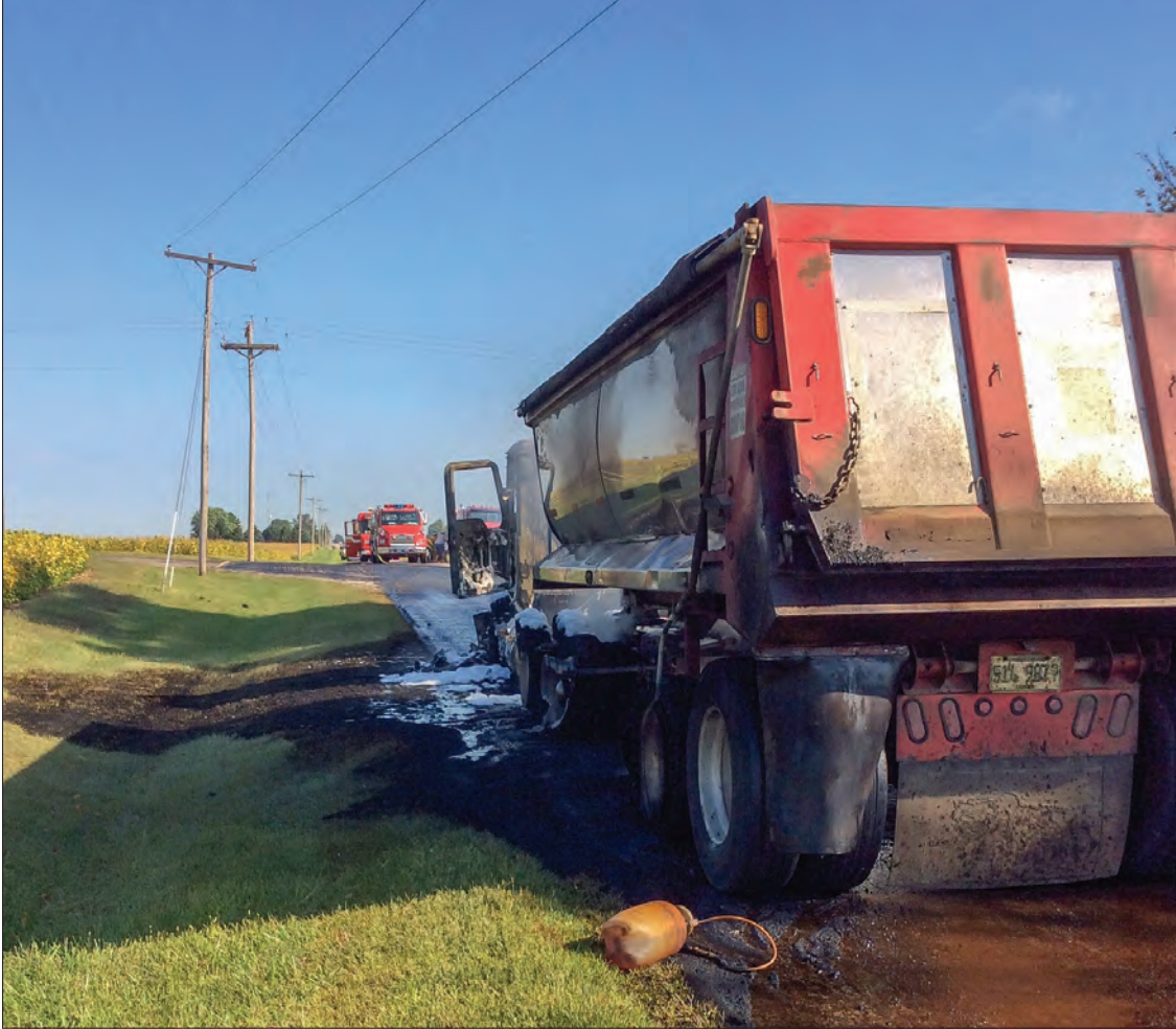
An Illinois asphalt truck operator raised the bed so he could clean the tailgate area, contacting the overhead power lines. Miraculously, the operator was shocked three times and survived. The truck, above and opposite page, was destroyed.
