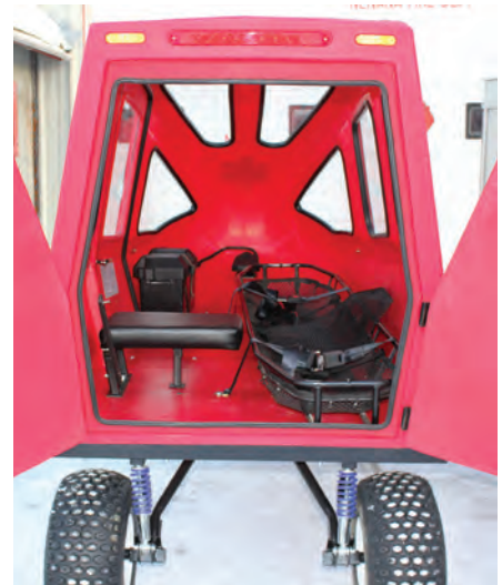
The SNOWbalance features a patient carrier, a seat for a medical technician and a small heater.
