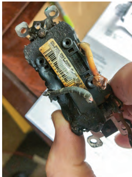
If your lights flicker and you smell burning plastic, call an electrician. This outlet was found thanks to an attentive homeowner.
