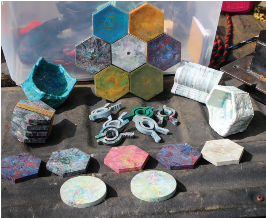
LEFT: Alan has made coasters, clips, flower vases and clock plates from recycled plastics. RIGHT: Byron Garcia, left, pours plastic pieces into the injection machine while Alan stirs the pieces as they melt. The melted plastic is pushed into a mold to create a coaster.
