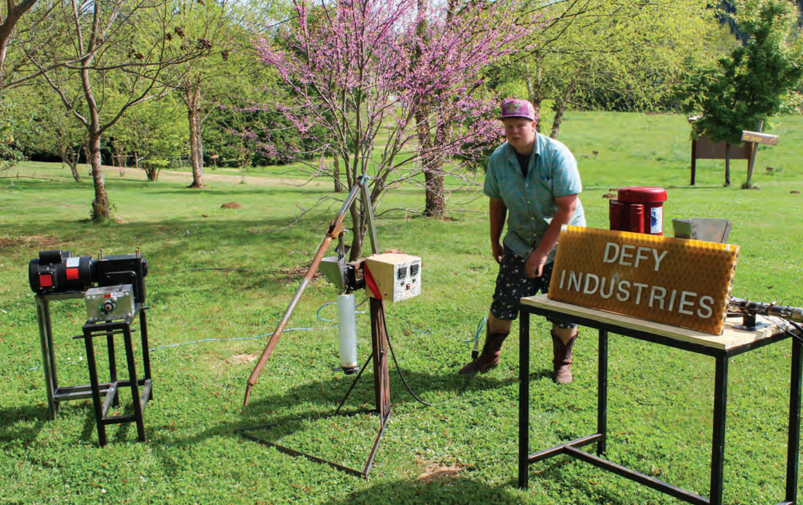
Alan Mooney, owner of Defy Industries, uses three machines—from left, a plastic shredder, an injection machine and an extrusion machine—to recycle used plastic into usable products such as coasters and clips.
