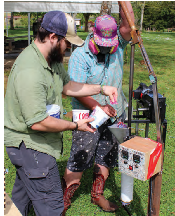
LEFT: Alan has made coasters, clips, flower vases and clock plates from recycled plastics. RIGHT: Byron Garcia, left, pours plastic pieces into the injection machine while Alan stirs the pieces as they melt. The melted plastic is pushed into a mold to create a coaster.
