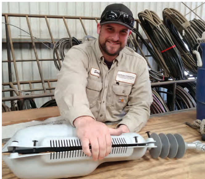
ABOVE: Lineman Sandy King demonstrates pole-top equipment covers that keep animals safer. OPPOSITE PAGE: Anza Electric is moving to ductile iron power poles for better fire resistance and strength.
