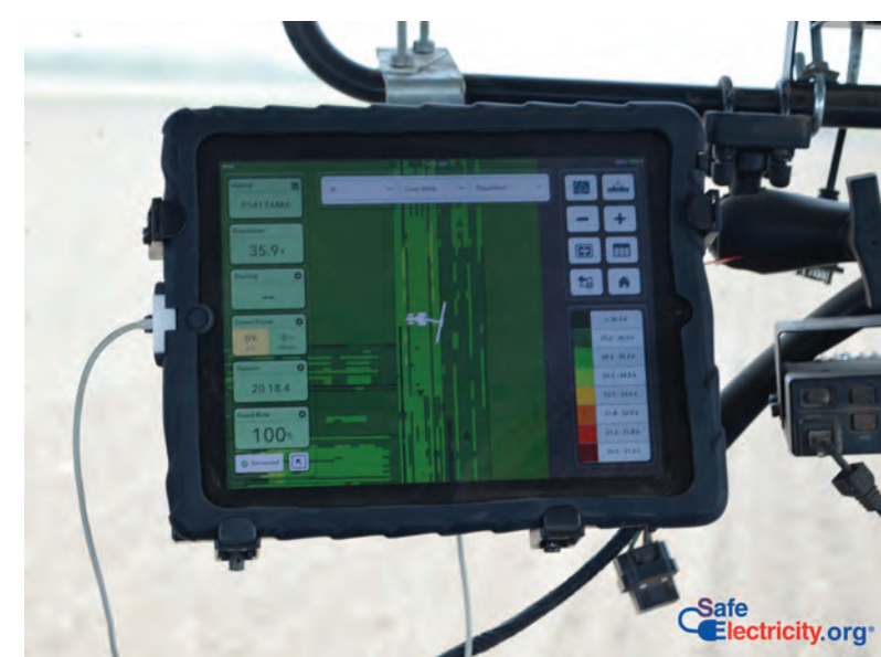
Thanks to GPS auto-steer devices, farmers are able to decrease driver error and maximize productivity. PHOTO COURTESY OF SAFE ELECTRICITY
