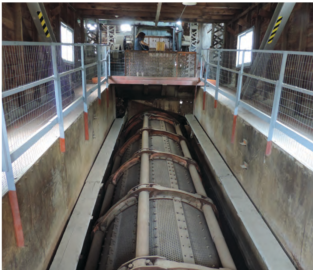
Inside the rotating trommel, where water was sprayed under high pressure to separate the gold and waste gravel.
